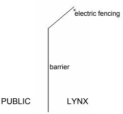
Figure 3: Barrier of a non-covered enclosure of the Eurasian lynx (pers. comm.)
